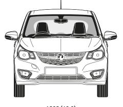
← 1595 (62.8) \_\_\_\_\_\_ excluding door mirrors ← 1876 (73.9) \_\_\_\_\_\_ including door mirrors
