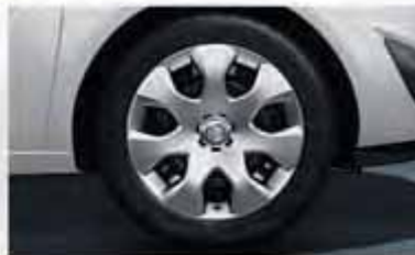
16-inch steel wheels with flush covers and 205/55 R 16 ultra-low profile tyres.
