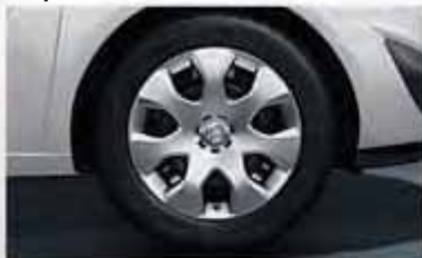
15-inch steel wheels with flush covers and 195/65 R 15 low profile tyres.
