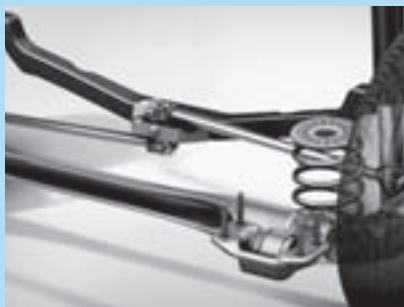
Watt's link improves handling and ride comfort.
