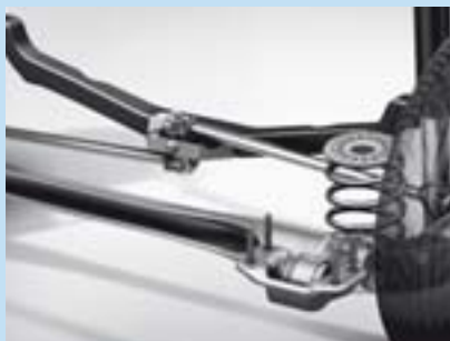
Watt's link improves handling and ride comfort.
