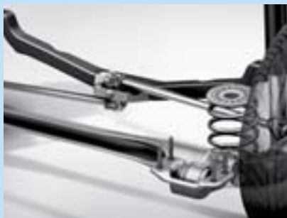
Watt's link improves handling and ride comfort.
