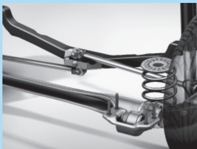
Watt's link improves handling and ride comfort.
