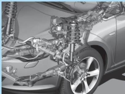
MacPherson strut front suspension.
