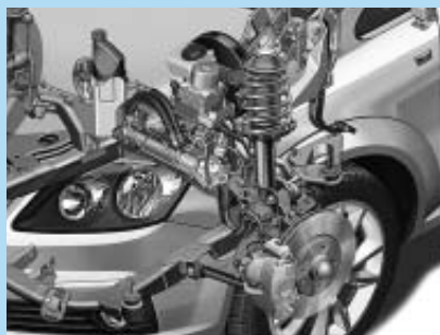
MacPherson strut front suspension.
