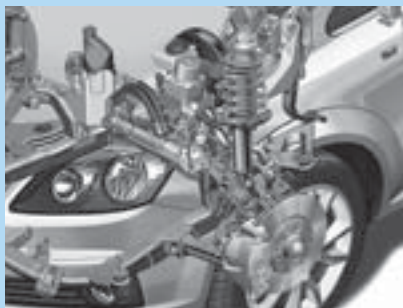
MacPherson strut front suspension.
