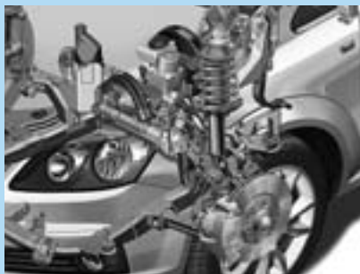
MacPherson strut front suspension.
