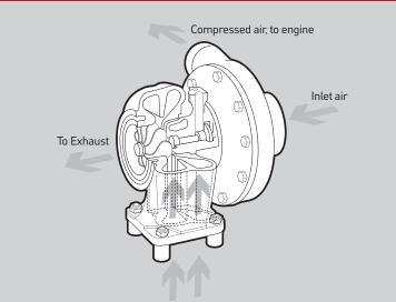
Exhaust gas, from exhaust manifold
