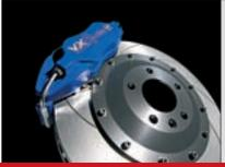
● Braking systems. For the driver who wants even more stopping power, VXRacing have developed, with AP Racing, a front braking system using four-pot calipers with larger diameter ventilated discs, high friction brake pads and braided hoses.
