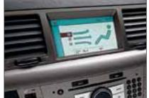
Electronic Climate Control (ECC). Flectronic Climate Control (FCC) allows you to select the temperature to the nearest degree and maintain it regardless of the outside temperature. The system, on some models, can even compensate for the effects of sunlight falling on one side of the car.
