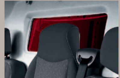
Bulkhead window A window for the steel bulkhead is available as an option, protecting the driver and crew while allowing an uninterrupted view of the cargo bay.
