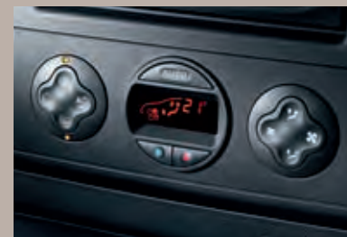
Electronic Climate Control Incorporates air conditioning and allows more precise, thermostatically-controlled temperature adjustment.
