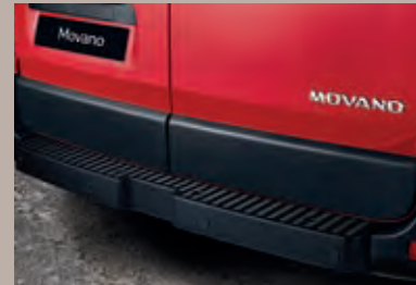
Rear bumper with integrated step Standard on RWD models, the rear step eases access to the load compartment. Optional on FWD models.
