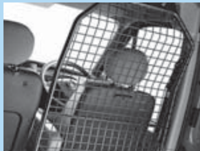
Full-height steel load restraint mesh behind driver.
