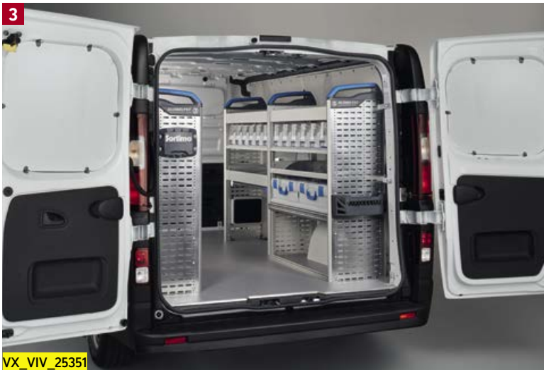
Model illustrated Vivaro L1 H1 fitted with Sortimo equipment.
