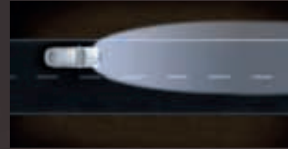
High beam with assist (any speed). Automatically switches from high to low beam as it detects oncoming or preceding vehicles.
