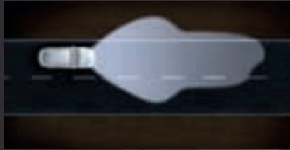
Motorway light (over 60mph). 140 metre range, higher and brighter than normal low beam without dazzle.
