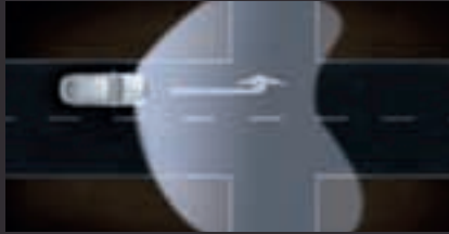
Pedestrian area light (up to 20mph). Wider spread of light (an extra eight degrees left and right) illuminates potential hazards.
