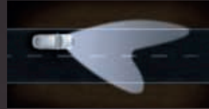
Country road light (30 – 60mph). Wider spread and brighter light than normal low beam. Longer illumination of own lane.
