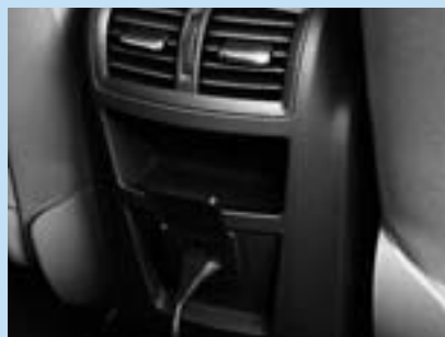
230-volt rear power outlet.
