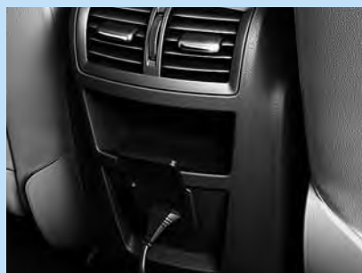
230-volt rear power outlet.
