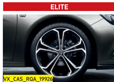
20-inch 5-spoke bi-colour alloy wheels with 245/40 R 20 tyres.**
