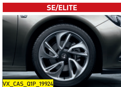
19-inch 5-spoke alloy wheels with 235/45 R 19 tyres.
