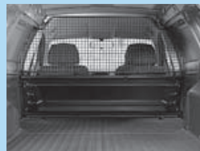
Upper load restraint mesh.
