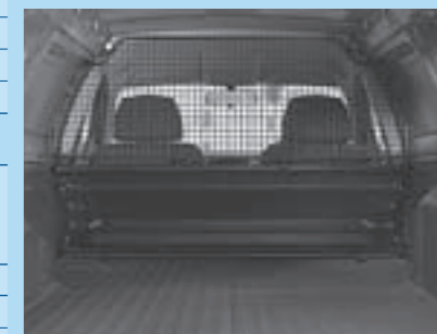
Upper load restraint mesh.
