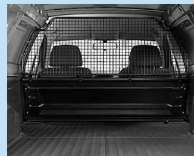
Upper load restraint mesh.
