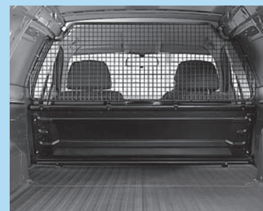
Upper load restraint mesh.
