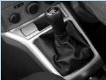
Six-speed manual gearbox.
