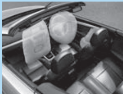
Front and side-impact airbags.
