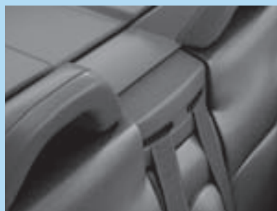
Two integral rear rollover protection hoops.
