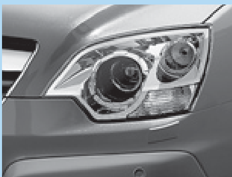
Xenon headlights with high-pressure washers.
