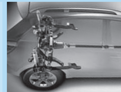
Rear suspension includes automatic self-levelling on 2.0CDTi 16v models.
