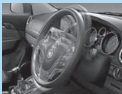
Steering column adjustable for reach and rake.
